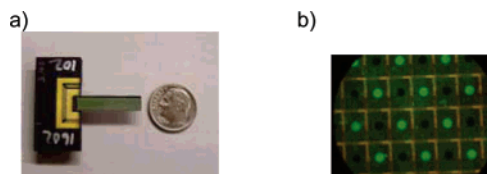
Figure 1. (a) A “1K-chip” having 1024 addressable electrodes in a 1 cm 2 area; (b) a chip utilizing the initially developed Wacker oxidation conditions at every other electrode. The ketone product was imaged by conversion into a 2,4-DNP derivative followed by incubation with a fluorescently labeled anti-2,4-DNP antibody. 5b
